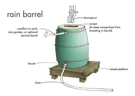
These rain barrels are typically arrayed to collect the run-off, from the roofs of various dwellings. Instead of using barrels, a community might simply direct the rain water towards shared cisterns or storage ponds. As with all water, you need to be aware of the possible contaminants, either from the atmosphere (acidity levels or other particulates in the water) or from the way the water is directed towards storage.
